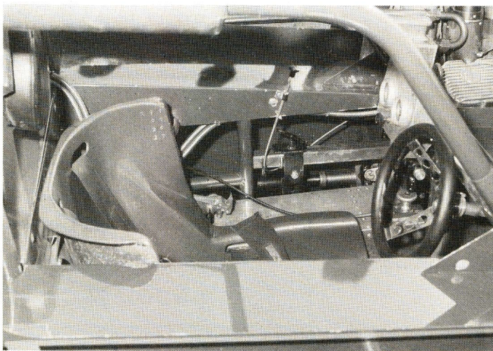
The adjustable torque arm and the fuel shut-off cable are just above the drive-shaft. The button controlling the in-out box is next to the steering wheel.
