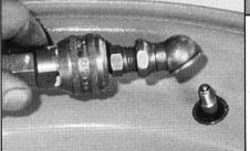
Apply R.T.V. silicon around the valve before inserting it in the hole.
