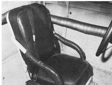
Driver protection sufficed with a single side bar in the roll cage. Side supports were welded on to the delivery van seat.
